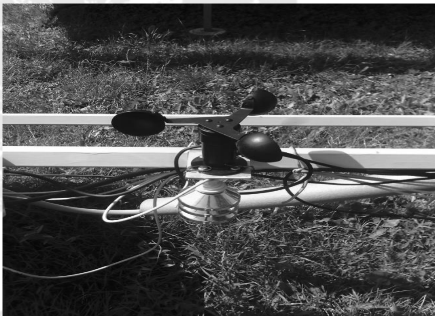
Figure 2. The wind speed sensor anemometer. (Zsiborács et al., 2016a)
